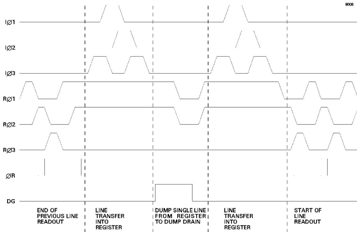
**FIGURE 9: DETAIL OF VERTICAL LINE TRANSFER (Multiple line dump)**
