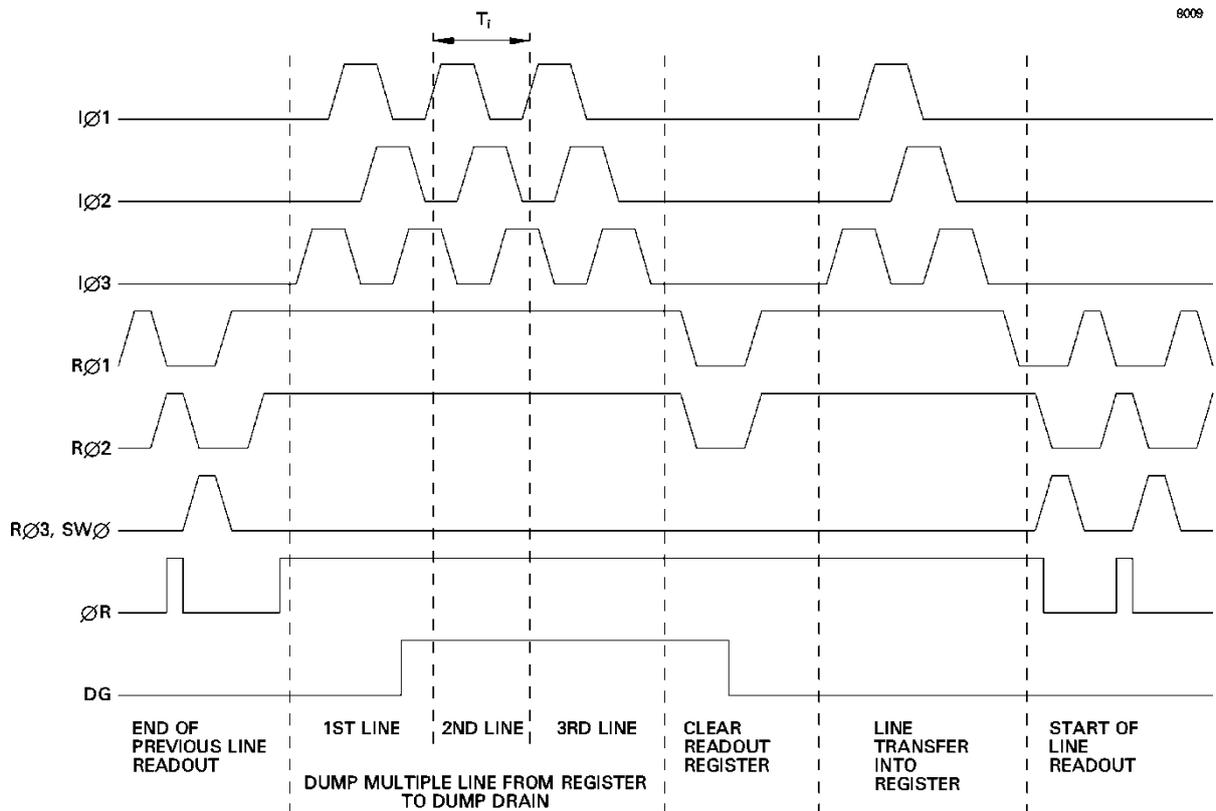
**FIGURE 10: DETAIL OF OUTPUT CLOCKING (Operation through both outputs)**
