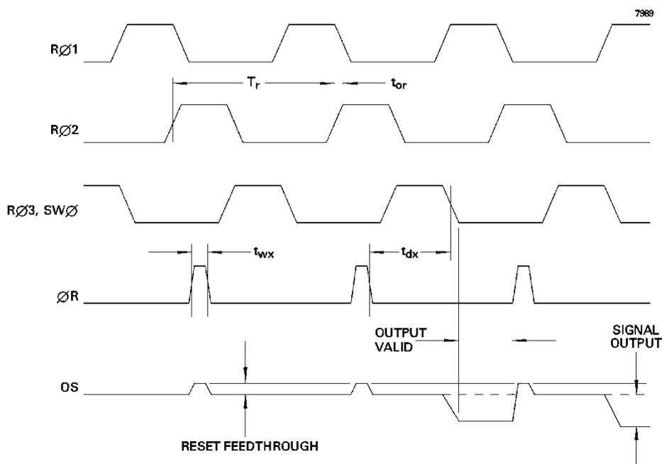
**FIGURE 11: LINE OUTPUT FORMAT (Split read-out operation)**
