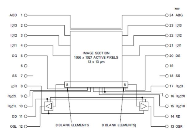
**Note** Pins 6 and 19 are not connected. For convenience, the CCD47-10 Compact Pack is pin compatible with the e2v technologies CCD57 sensors in the compact pack, except that OSL = pin 6, OSR = pin 19 and pins 12 and 13 are not connected in the CCD57.
