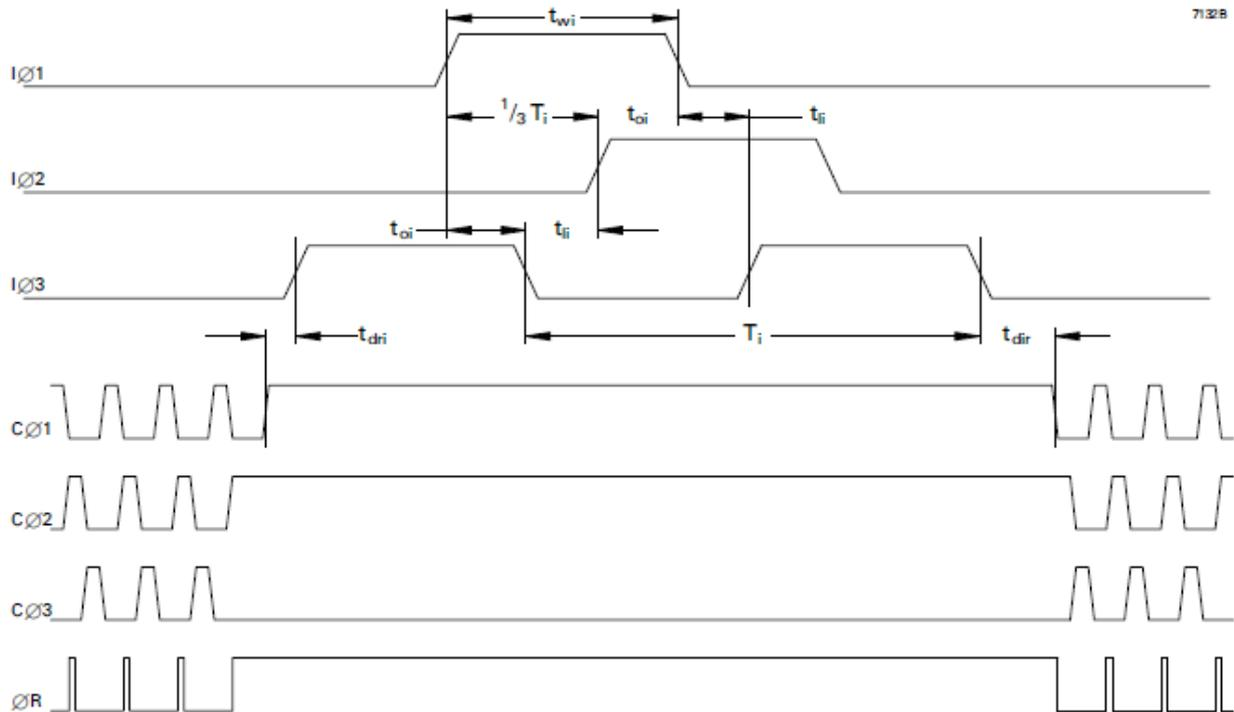
**Note:** For Full Frame readout,  $IØ = AØ = BØ$ . For Frame Transfer,  $IØ = BØ$  whilst  $AØ$  is low for charge collection.
